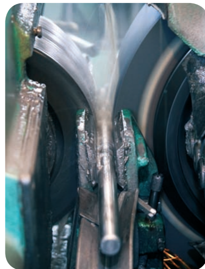
Pins are ground to thoroughly optimize the wear life.
