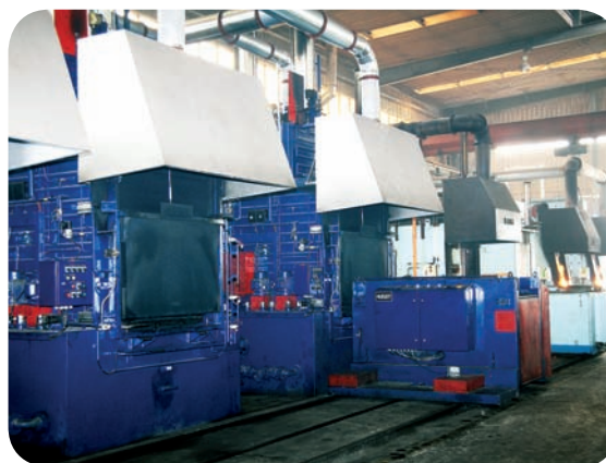
Furnaces for heat treatment process
