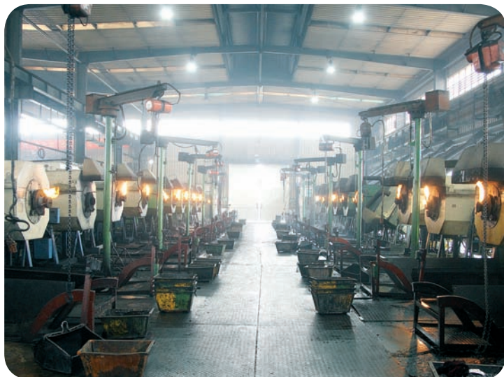
Rotary furnaces are used for pin heat treatment to ensure uniform heat dispersion.
