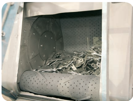
Shot peening parts improve fatigue and crack resistance
